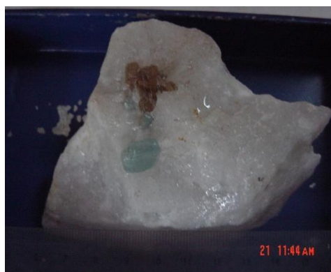
Figure 16. Apatite in marble associated with phlogopite mica board of Myasein Taung area, Momeik Township.
