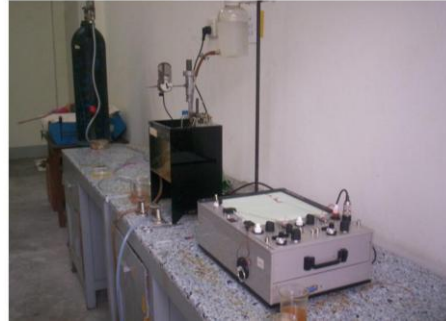
Figure 4. Apparatus set used (2 channel recorder GEMIN 7070, organ bath, water jacket, O 2 cylinder & pipe)
