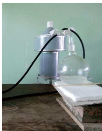
Figure (2) Steam distillation apparatus
