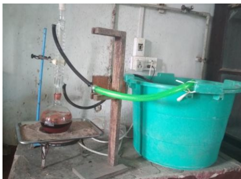
Figure (3) Extraction of Cellulose Pulp from Stem Wood Powder of Tamalan
