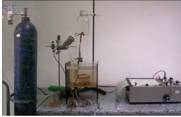
Set up of apparatus for isolated rat uterus preparing
