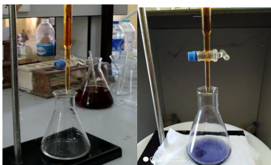
Figure 3. Experiment for Iodometric Titration
