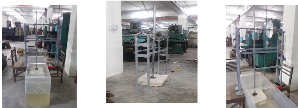
Figure 3 Wave generator assembly
