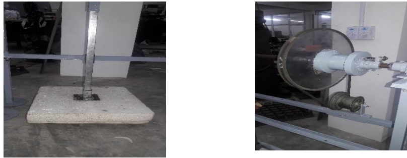
Figure 2 Buoy (floating device), pulley, belt and dynamo of wave generator
