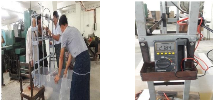
Figure 4 Preparation for wave energy generator assembly with setup and testing by wave
