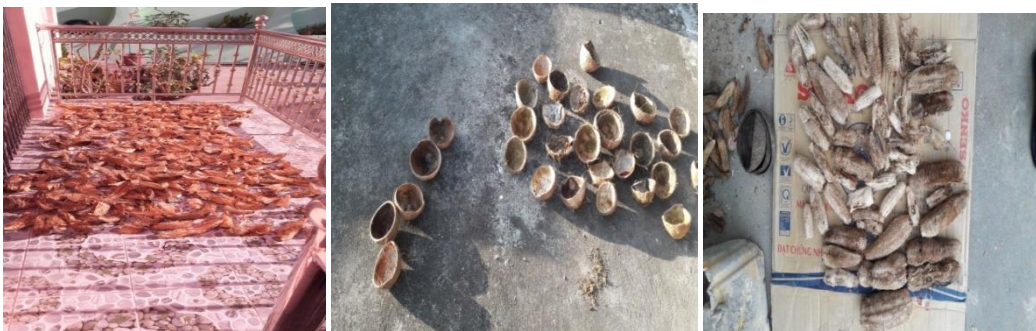
Figure 3 Sample preparation( drying) of coconut shell coir ,coconut hard shell and loofah by heating process
