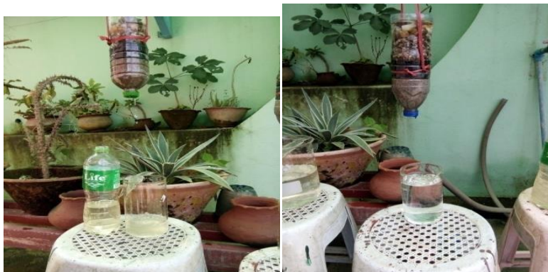
Figure 7 Water filtration process for rural area application
