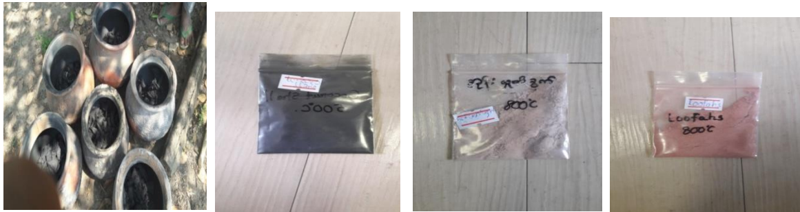
Figure 5 Sample of activated carbon by coconut shell coir and coconut hard shell at temperature 500° C
