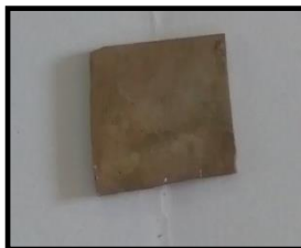
Figure 3. Ag- \text{TiO}_2 thin film annealed at 600 °C
