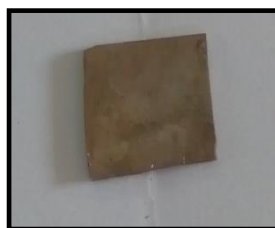
Figure 3. Ag-TiO 2 thin film annealed at 600 °C
