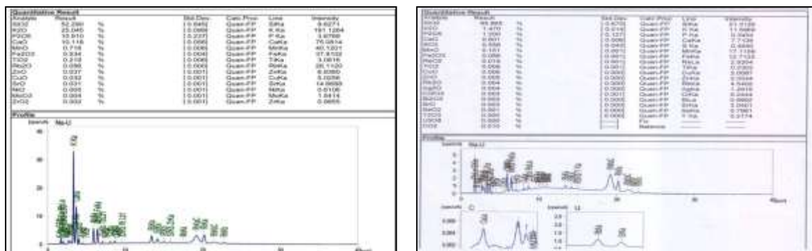
Figure 1 EDXRF spectra of BLA and RHA
