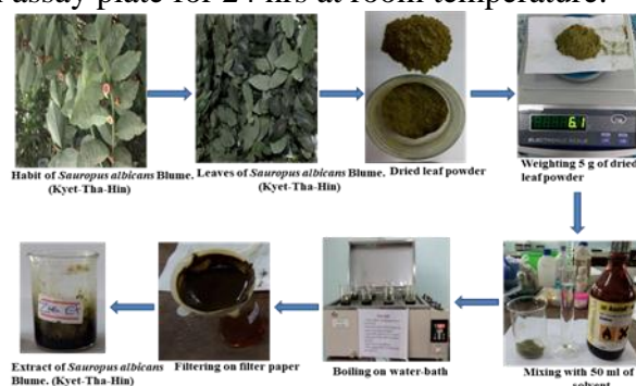
Fig 1. Procedure for the extraction from the leaves of Sauropus albicans Blume. (Kyet-Tha-Hin)
