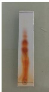
Figure 2. Separation of Amino Acids from Sample Solution (Ethanol Extract, Crude) by Thin-Layer Chromatography
