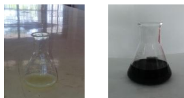
Figure (7) Titrimetric Result of 10 ml of Sample Solution of Fresh Fruits with 0.0051 M of Iodine Solution
