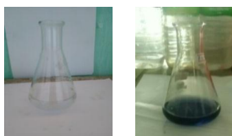
Figure (6) Titrimetric Result of 10 ml of 0.0057 M Standard Ascorbic Acid with Iodine Solution
