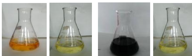
Figure (4) Titrimetric Result of 10 ml of Sample Solution of Fresh Fruits with 0.0465M of Iodine Solution
