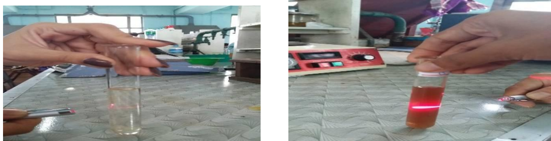
Figure 3. Photograph of confirmation test for presence of nano colloids by Tyndall effect
