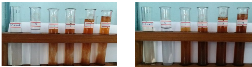
Figure 2. Before and after addition of Ixora coccinea L. leaf extract into \text{AgNO}_3 solution
