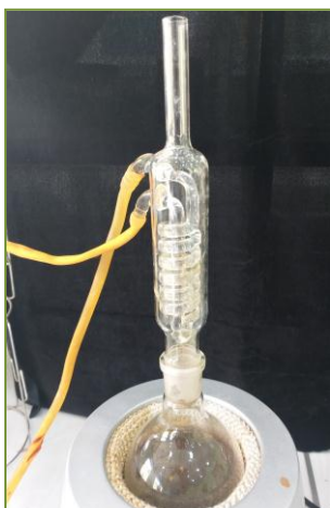
Fig.2 Extraction of mucilage by soxhlet extractor
