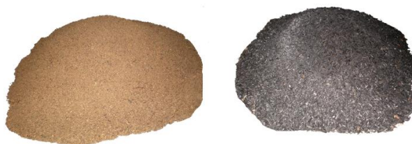
Figure 1. Photograph for (a) Rice husk ash (from brewery factory) (b) Tea residue
