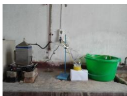
Figure 3. Steam distillation apparatus Figure 4. Essential oil Figure 5. TLC check
