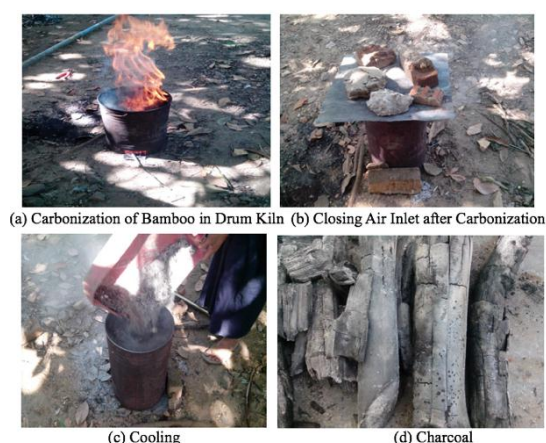
Fig.2 Stages of White Charcoal Processing Using a Drum Kiln
