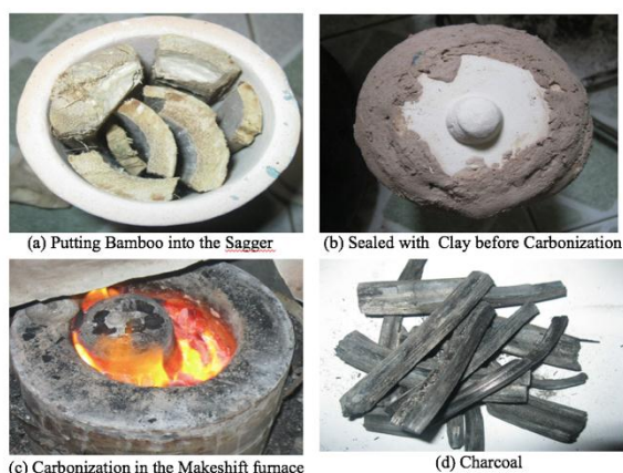
Fig.4 Stages of White Charcoal Processing Using a Makeshift Furnace
